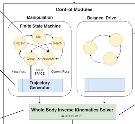
Trajectories interpolate a smooth path between target states
