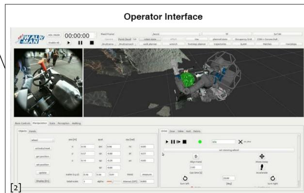
A simulated environment allows selecting target objects and locations
