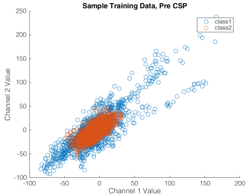
Figure 6: Muse Headset Data showing difference between Open Eyes(Class 1) vs Closed Eyes(Class 2) before CSP is applied
