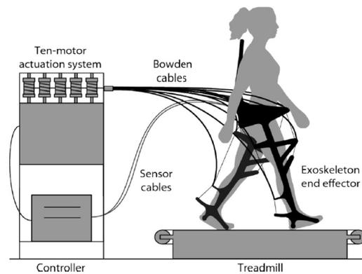
**Figure 1.** Schematic of hardware system (Bryan et al. 2020). The ten-motor stand actuates hip flexion/extension, knee flexion/extension, and ankle plantarflexion via Bowden cable transmissions.
