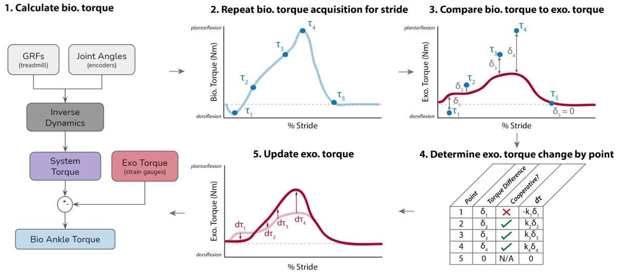
**Figure 2.** High-level exoskeleton control strategy using a biological torque based heuristic.
