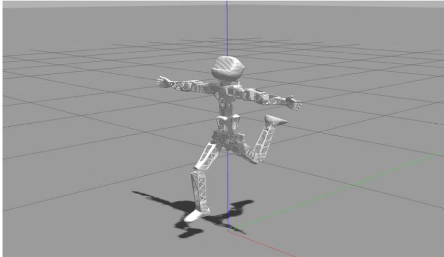
In addition to this visual confirmation in Gazebo, we can check that Poppy's joint positions are changing by subscribing to the ROS topic `joint_states`. The command `rostopic echo /joint_states` outputs a continuous stream of joint positions, velocities, and efforts.
