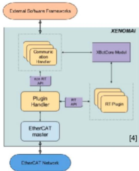
Given its high transmission rate, XBotCore was originally designed for EtherCAT based robots. However, later versions of the software support any device driver via a hardware abstraction layer<sup>1</sup>.
